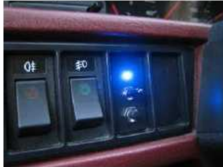
Picture of Flexitune command panel in a Volvo with LED, 3-way switch and pushbutton
