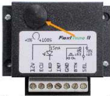
Remove potentiometer Cap for adjustment
